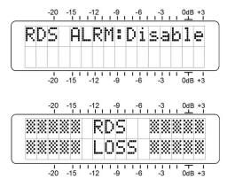
Select FI Err. for the 633 to give an alarm for a PI code mismatch between the received PI and the PI code entered into the 633 by the user. (Instructions for entering the PI
