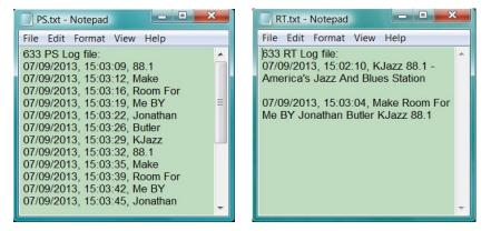
Note that the PS log shows frequent updates. This is because the PS message is *dynamic*, or scrolling. Scrolling-PS essentially creates a new 8-character display every few seconds. The Radio Text field, on the other hand, shows only a single update during the example logging period, a station promo replaced by title and artist once the song started.
